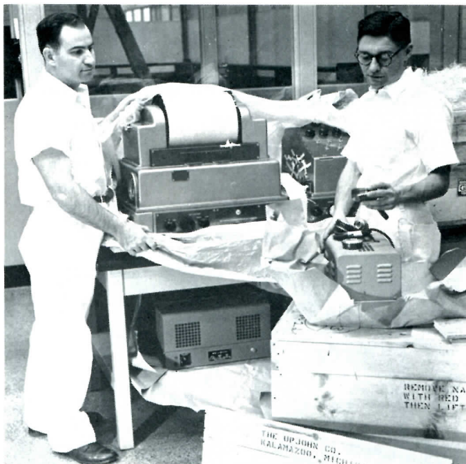
The Infra-red Spectrophotometer, which Marv Grostic and Bill Bartelt unpack, is an important addition to the list of Control Lab instruments. Marv spent three months in the Department of Physics learning to operate this highly specialized instrument. Bill is usually in lab across corridor from this one where he does analysis via paper chromatography.
